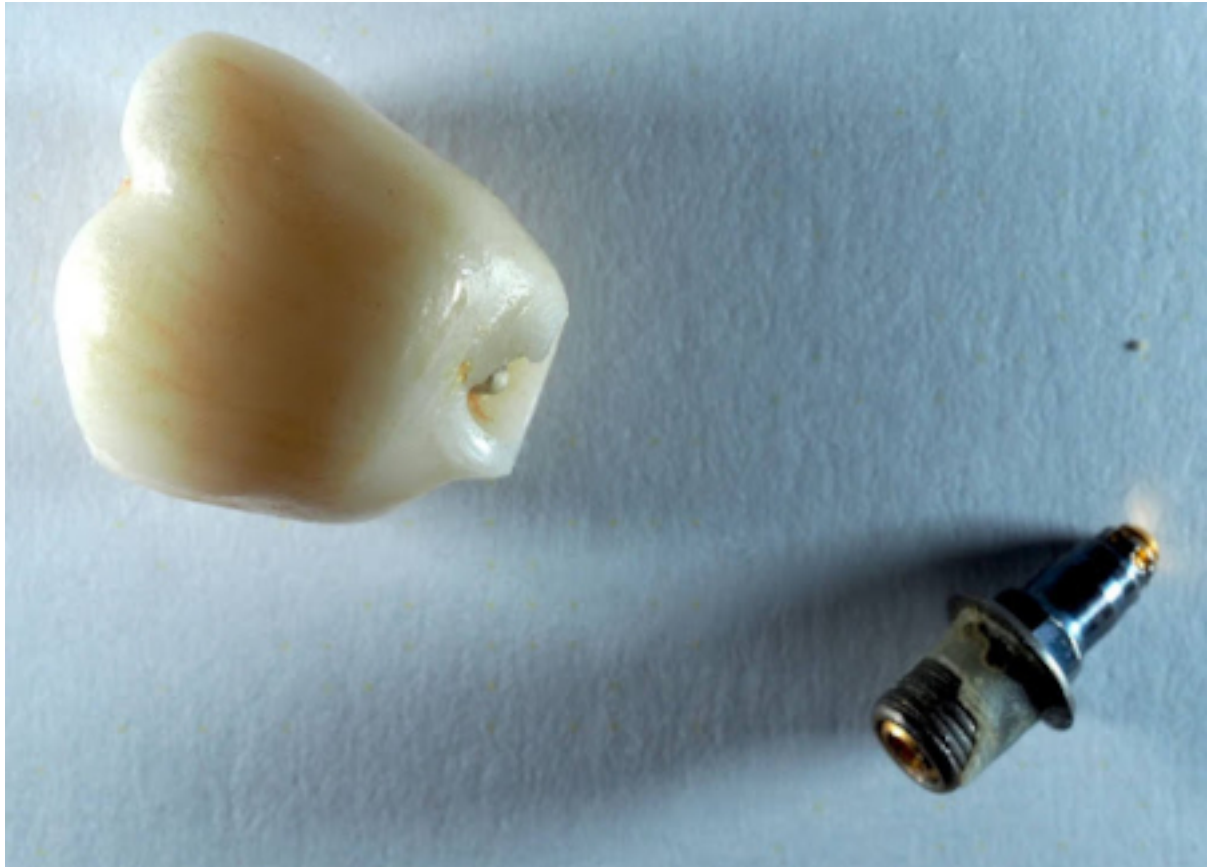
Figure 6: An example of a fracture of dental implant components
